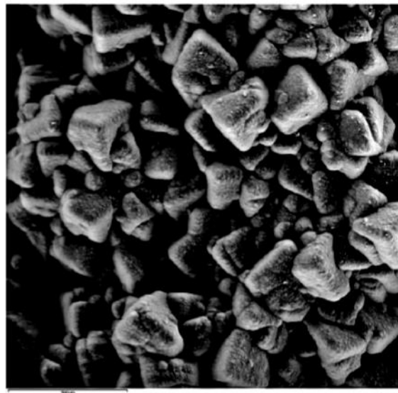
Figure 6. Scanning electron microscope image of quartz in figure 5 from the Penn/MD Materials quarry. Magnification is approximately 163X.
