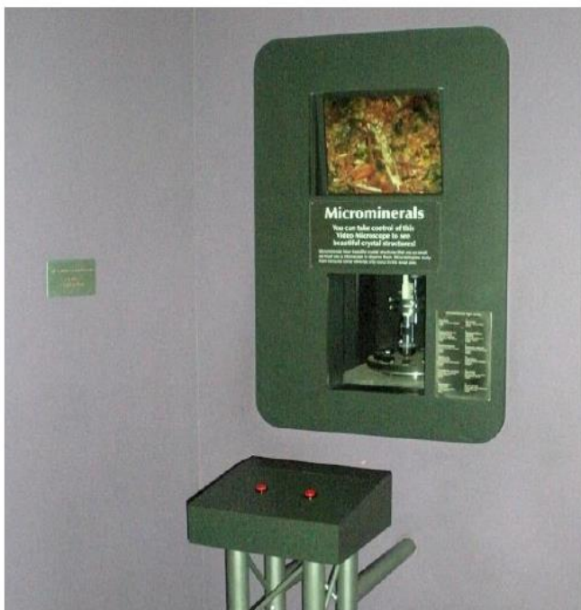
Figure 1 The Cleveland Museum of Natural History's micromount display, features the micromounts on a turntable and a microscope with a video camera feeding the video screen allowing viewers to choose the specimen and its magnification.
