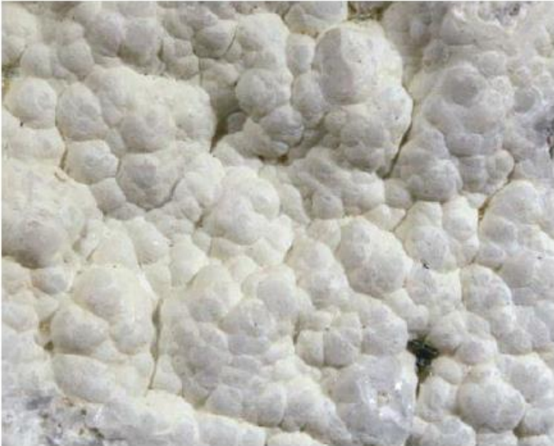
Figure 12. Quartz-magnesite mixture from the Penn/MD Materials quarry; close-up of specimen in figure 11, showing cracks in surface. Field of view is 1.3 cm.
