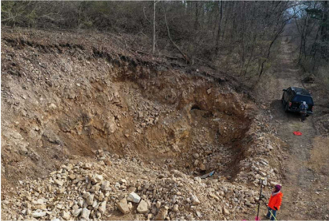
Photograph 1. of the Westerly (Upper) Wavellite Adit/Pit. Previously existing spoils that were used to build up and berm the road. New spoils that do contain specimens of Wavellite overlooked during the exploration. The active workings extend below the cardboard box easterly into the wall. The westerly side of the pit contains no Wavellite. Wavellite extends from the lower left (westerly, exposed) shoulder of the excavation to 3 feet off the southerly wall (road), down about 16 feet and easterly toward the easterly pit.
